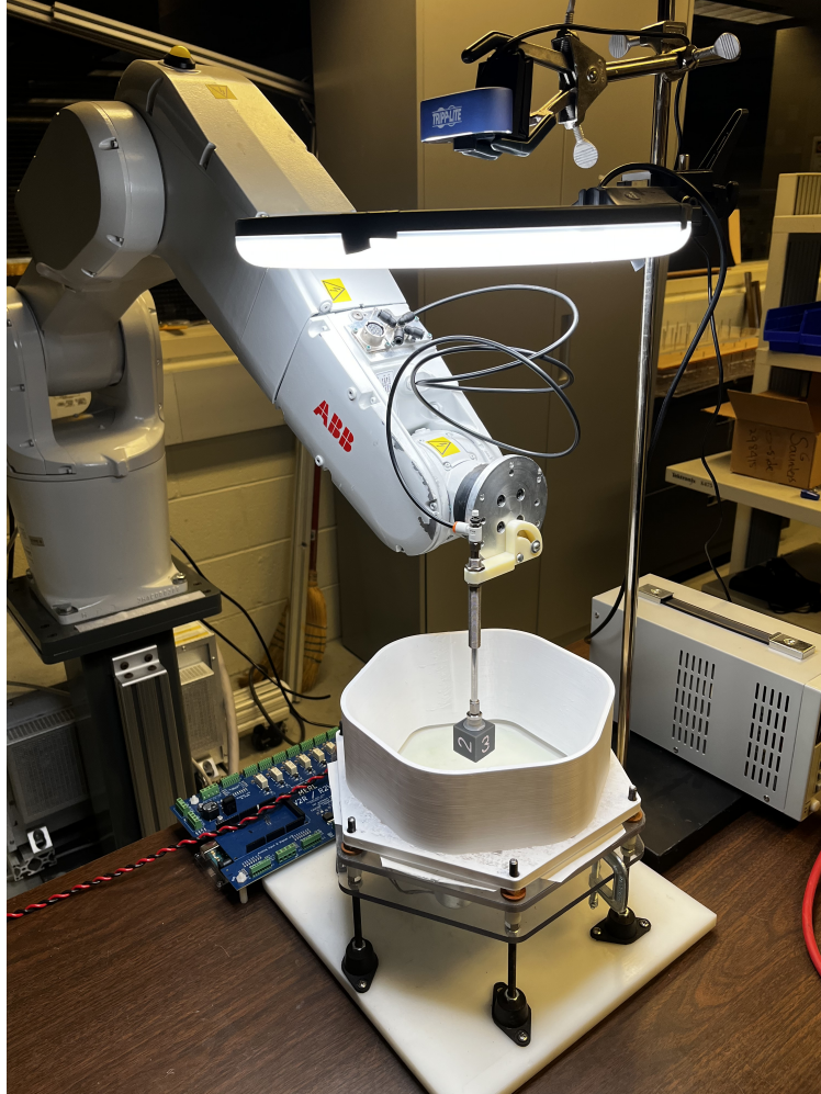
Figure 6.1: Thumper joined with an ABB IRB 1200 Robot Manipulator holding a die with a suction cup
