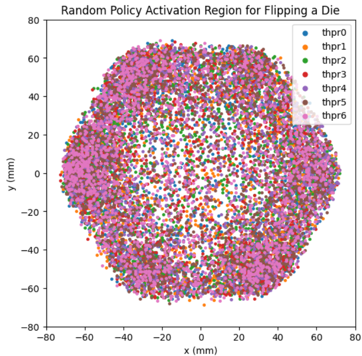
Figure 4.15: Random Policy: Die positions and the solenoid fired.
